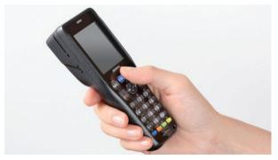
barcode. When the barcode has been read successfully, the terminal will beep and the blue indicator LED at the top of the screen will flash briefly.
