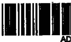
High Resolution with bars touching due to bleed and insufficient spacing
